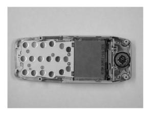
**10.** Gently place the LCD module into its place.
