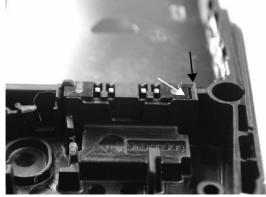
**6.** The battery connector will be assembled into the D-cover with interference fit.
