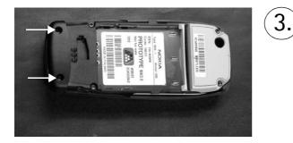
) Remove the screws from the bottom end with specified tool.
